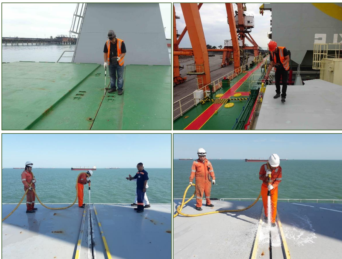
Pictures 21 to 24: Hatch covers ultrasonic test (above) and hose test (below). Source: Proinde
