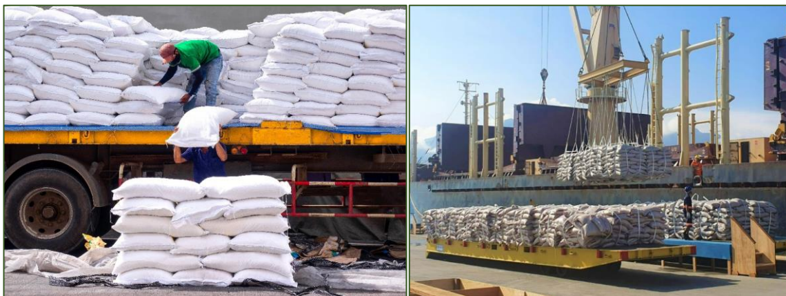
Pictures 13 & 14: Loose bags being placed on slings (left) and pre-slung bags being loaded. Source: Shutterstock/Proporto
