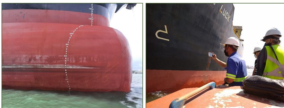
Pictures 29 & 30: Cargo quantification by draft survey. Source: Proinde
