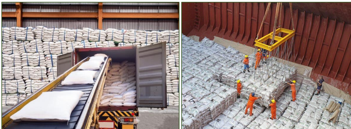
Pictures 15 & 16: Loose bags being stuffed into a container and pre-slung bags being stowed. Source: Shutterstock/Proporto
