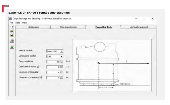
The "BVLash" software is available and can be used to calculate lashing as per CSS code.
